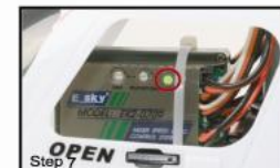
Step 7 Permanent light of green light is ready to fly 绿灯恒亮即显示待飞
