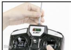
Step 3 Draw out the antenna of transmitter completely 完全抽出发射机天线
