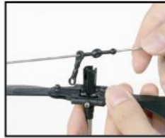
A 平衡杆拆卸 Stabilizer set disassembling
