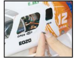
E 机壳拆卸 canopy disassembling
