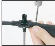
C 主旋翼拆卸 Plastic blade disassembling
