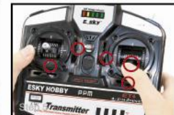
Step 5 Set the throttle stick and the throttle trim to the lowest position and other trims to the center point 把油门摇杆和微调调至最低, 其他微调定位在中心点。
