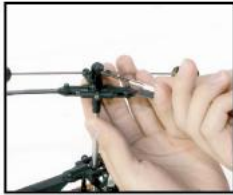
A 平衡杆拆卸 Stabilizer set disassembling
