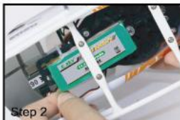
Step 2 Put the battery into the battery holder 将电池装入电池架
