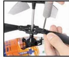
C 主旋翼拆卸 Plastic blade disassembling
