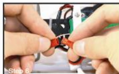
Step 6 Plug the battery into the battery lead of 4-in-1 wint 接通直升机电源
